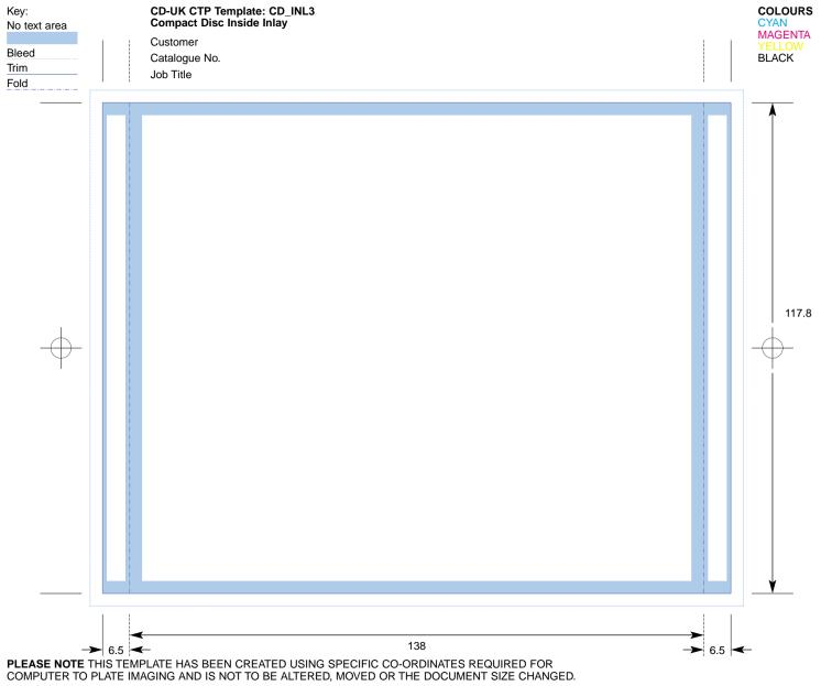
ALL DIMENSIONS ARE IN MILLIMETRES. BLEED ALLOWANCE OF 3MM ON TRIMMED EDGES
