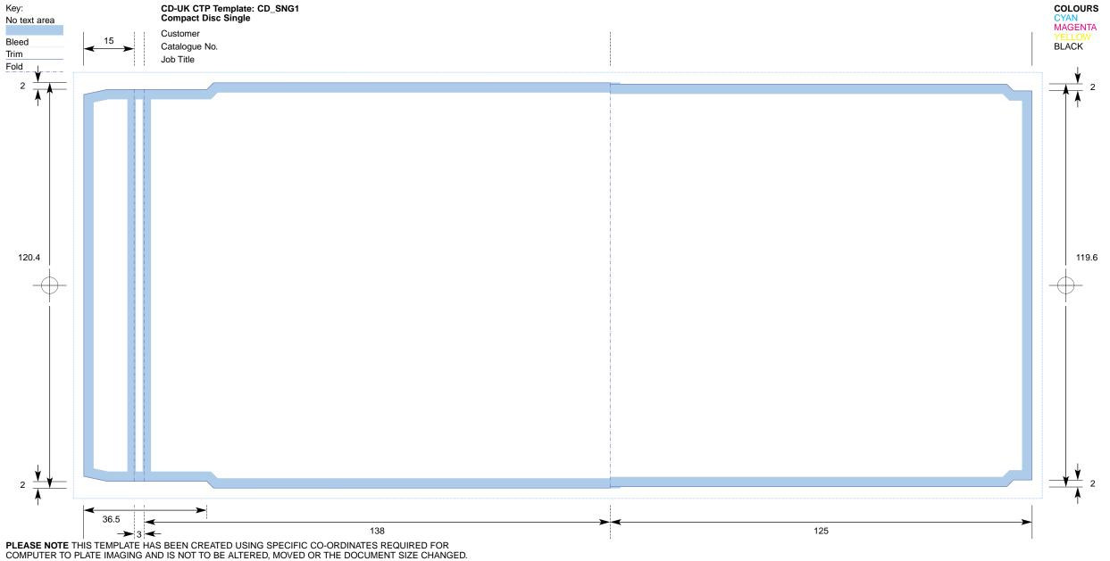
ALL DIMENSIONS ARE IN MILLIMETRES. BLEED ALLOWANCE OF 3MM ON TRIMMED EDGES
