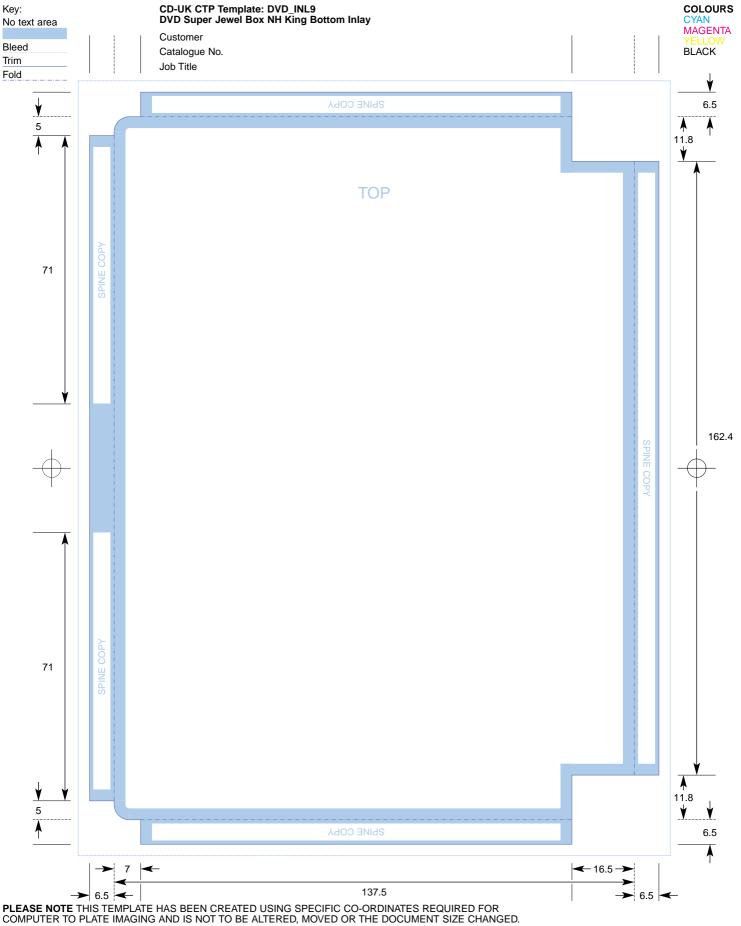
ALL DIMENSIONS ARE IN MILLIMETRES. BLEED ALLOWANCE OF 3MM ON TRIMMED EDGES
